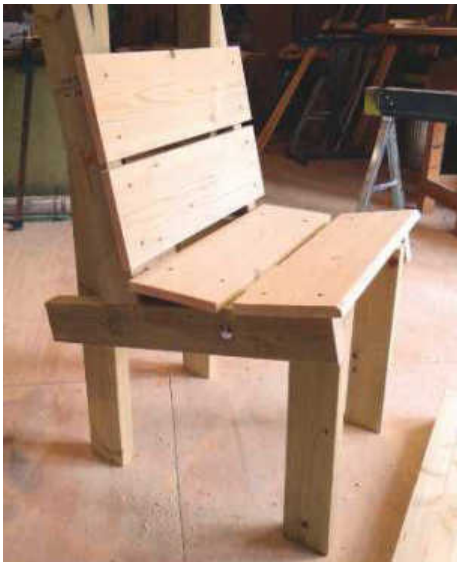
PIC 7. With just one bolt in place, the secondary frame can be swivelled just a little to ensure that the planks fit the angled back
